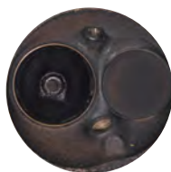
Cylinder head before P.i. treatment.
