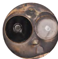
Cylinder head after one P.i. treatment.
